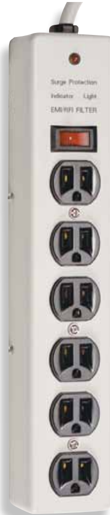
91-222 4' Cord 6 Outlet Professional Metal Surge Strip, 540 Joules 15A-120V, 1800 W Packing: 12/Master
